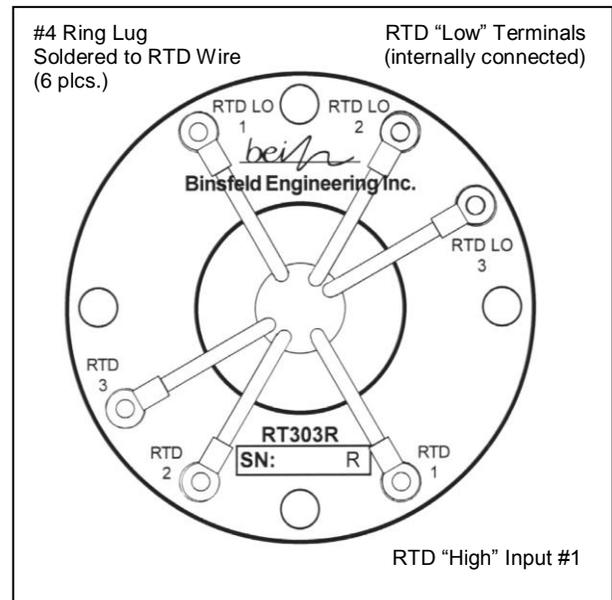
Rotor/RTD Wiring Diagram
