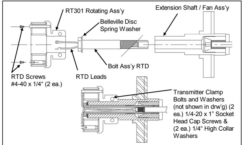
Bolt & Rotary Ass'y Installation Diagram
