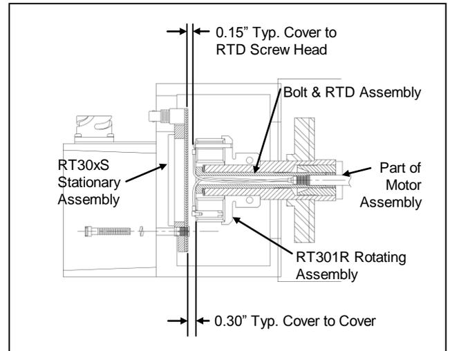
Completed RT301 Installation Diagram
