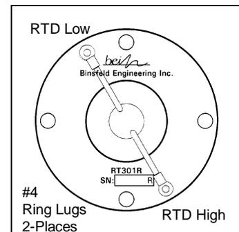
Rotor/RTD Connection Diagram
