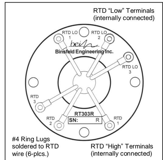
Rotor/RTD connections Diagram
