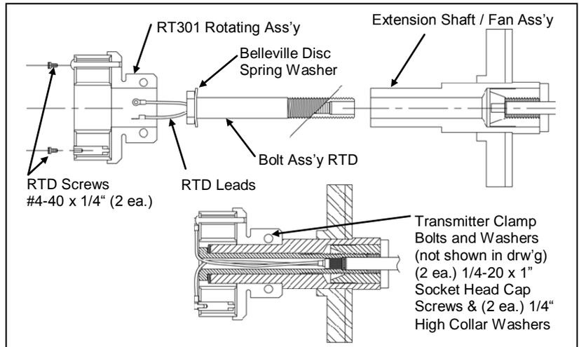
Bolt & Rotary Ass'y Installation Diagram
