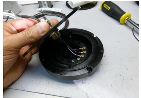
Fig. 6 – Stator Top Plate with Gland
