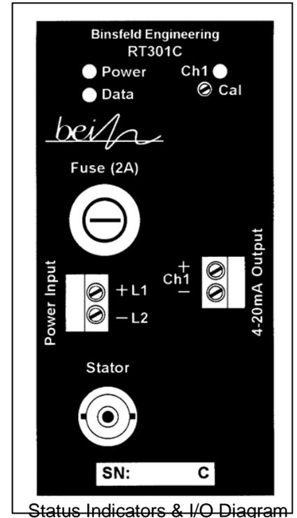
If the status lights do not agree with conditions listed above, remove power to the RT301C for 5 seconds, and then restore power (to reset the digital circuitry). Go to <http://www.binsfeld.com/temptrak/rt300/> for more trouble shooting aids.
