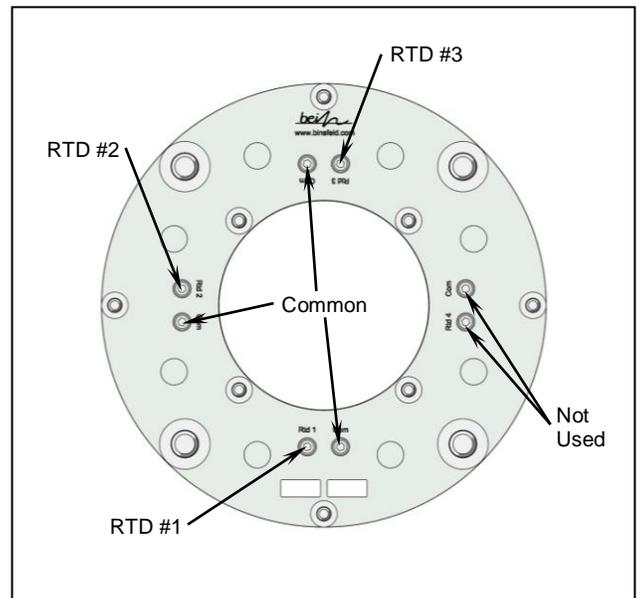
Rotor/RTD Wiring Diagram
