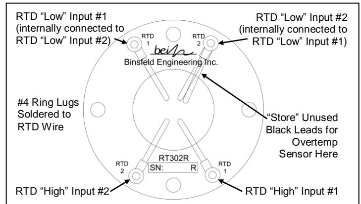
Rotor RTD Wiring Diagram
