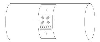
Positioning the Gage on the Shaft
