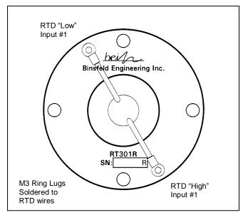
Rotor/RTD Connections Diagram
