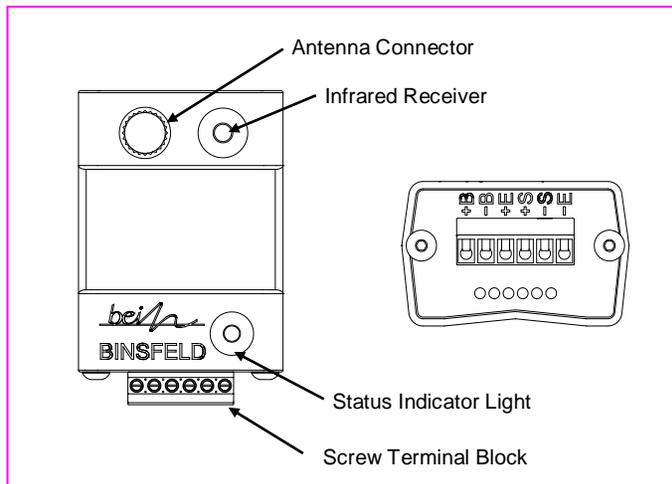
**Figure 3: TX10K-S Transmitter**
